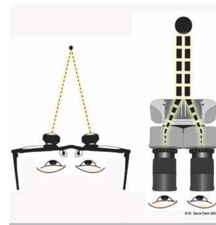
Figure 9 Oculars (loupes) rely on convergent vision that essentially requires an overlap of two images. This form of magnification creates increasing problems and eye strain as magnification power increases. The clinical microscope uses a more refined optical system.
